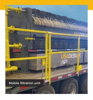
Closed-Loop filtration is an optional feature of USA DeBusk's pigging and decoking service. As part of a self-contained system, the filtration unit operates continuously during the decoking process to remove and capture entrained particulates from the effluent and provide clean water for nonstop decoking. The filtration unit has a compact footprint and increases the overall safety and environmental sustainability of the pigging process.
